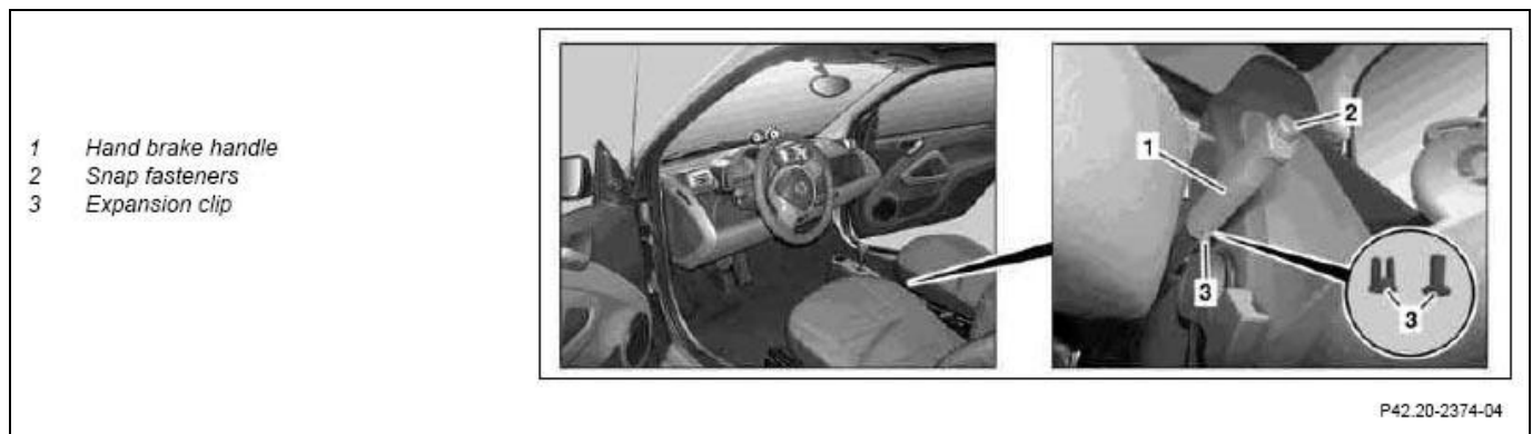
Fig 1: Identifying Hand Brake Handle, Snap Fasteners & Expansion Clip
