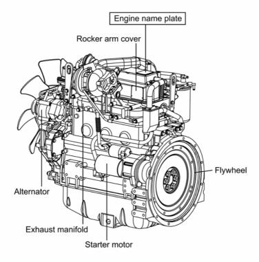
Note) • This illustration shows the 4TNV98T engine (with turbocharger).
