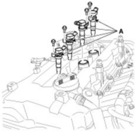
Fig. 2: Identifying Ignition Coils Courtesy of KIA MOTORS AMERICA, INC.
