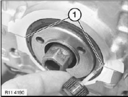
**Fig. 78: Coating Surface Of Sealing Compound In Both Grooves With Loctite Primer**
