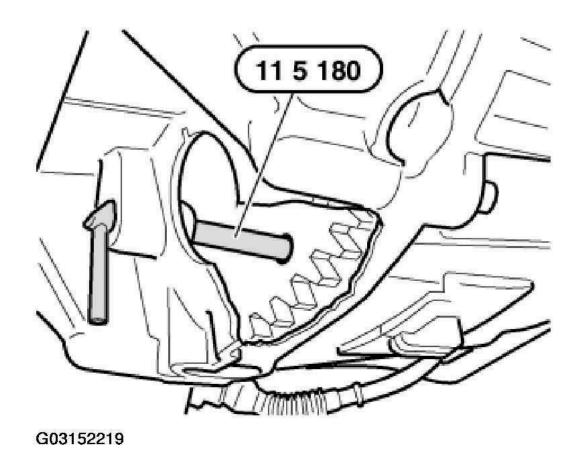
Fig. 322: Holding Crankshaft With Special Tool 11 5 180 In TDC Firing Position Of First Cylinder Courtesy of BMW OF NORTH AMERICA, INC.
