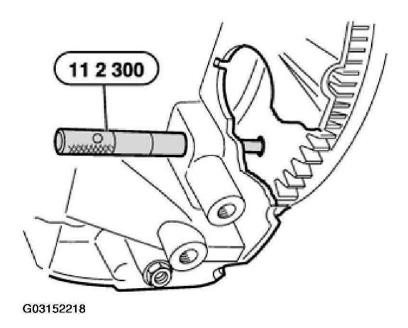
Fig. 321: Holding Crankshaft With Special Tool 11 2 300 In TDC Firing Position Of First Cylinder Courtesy of BMW OF NORTH AMERICA, INC.
