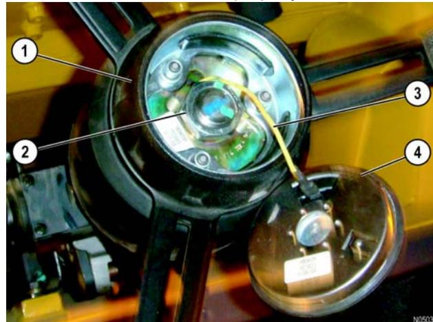
FIGURE 5-3. STEERING WHEEL RETAINER NUT
