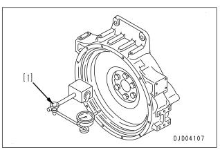
Install the output shaft assembly. For details, see "Removal and installation of output shaft assembly".
