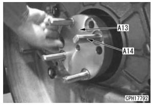
2] Insert tool A16 into tool A13, adjust the position of tool A13 so that the centers of crankshaft (4) and tool A13 are aligned, tighten tool A14, and fix them.
