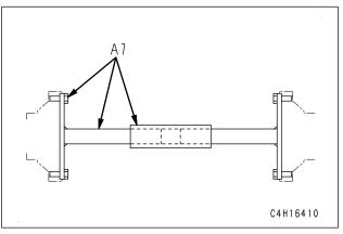
Mounting bolt for drive shaft between engine and transmission: Loctite (LT-2)
