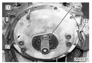
19. Remove output shaft assembly (28) by using forcing screw [1] and guide bolt [2].
