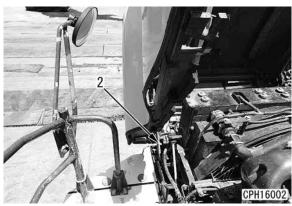
Tilt up operator's cab assembly (3). For details, see Testing and adjusting, "Cab tilt up procedure".
