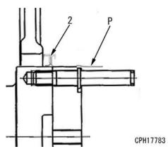
7] Put tool A18 (bolt: stem length 60mm) through to tool A15, and insert tool A17 (spacer) to tool A18.
