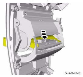
5. Install and tighten the two screws that attach the holder for the navigation display screen to the mechanism for the navigation display screen.
