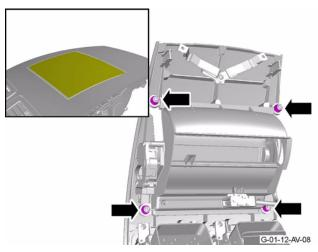
12. Tighten the four screws that attach the mechanism for the navigation display screen to the veneer bezel.
