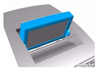
3. Install the holder for the navigation display screen to the two clips that attach it to the mechanism for the navigation display screen.
