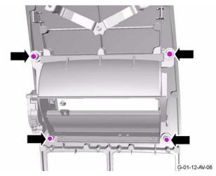
13. Install the veneer bezel for the IP (Refer to Workshop Manual procedure 01.12.AV - Veneer Bezel for the Instrument Panel (IP)).
