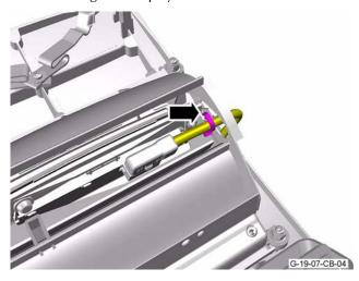
Manually move the navigation display screen into the closed position.
