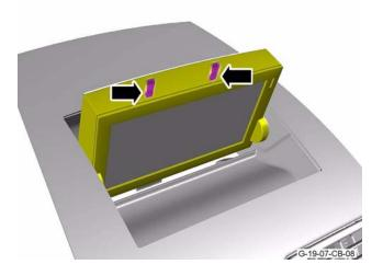
4. Install the holder for the navigation display screen to the mechanism for the navigation display screen.
