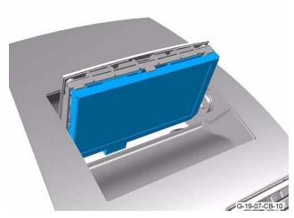
2. Put the holder for the navigation display screen into position.
