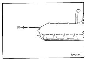
Remove the spring and pressure regulator plunger.
