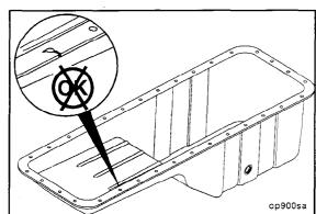
Visually inspect the oil suction tube and brace for cracks. Do not reuse a cracked oil suction tube or brace.
