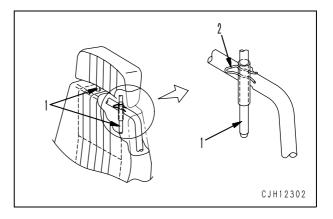
Apply force (b) to part (a) of each clip (2) in the direction of the arrow to turn the clip. Release headrest stay (1) from part (d) of the clip and pull out up headrest (3).
