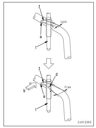
★ Pushing in both clips (2) simultaneously, remove headrest (3).
