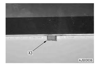
2) Using styrene foam blocks [9] and rubber bands [10], fix the window glass and both-sided adhesive tape for at least 10 hours to fit them completely.
