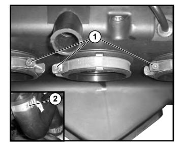
Loosen the screws of the clamps (1) on the throttle bodies. Take off the elastic clamp (2) take off the pipe
