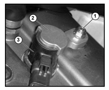
Loosen and remove the nut (1). Remove the coil support rod (2), Slip off the coil. Remove the sparking-plugs beneath.
