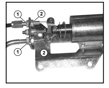
Loosen the nut (1) and the lock nut (2). Take off the recall cables, take off the connector, remove the solenoid.
