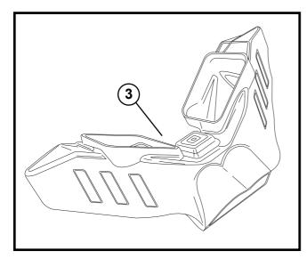
Take off the Air Box base disconnect the air sensor connector below it. Remove the Air Box air duct (3). Check the state of the components visually, if necessary replace
