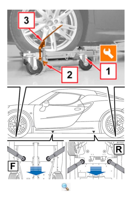
Due to the high sportiveness of the Alfa 4C, special attention should be paid to the lifting with the arm lift, to all procedures involving car handling including the loading/unloading from the car transporter/breakdown truck, travelling on ramps and humps, etc. Fig. 18 and the relevant table hereby give the following values:
