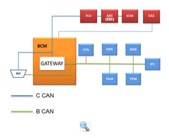
The electronic control units sharing data on C-CAN are:
