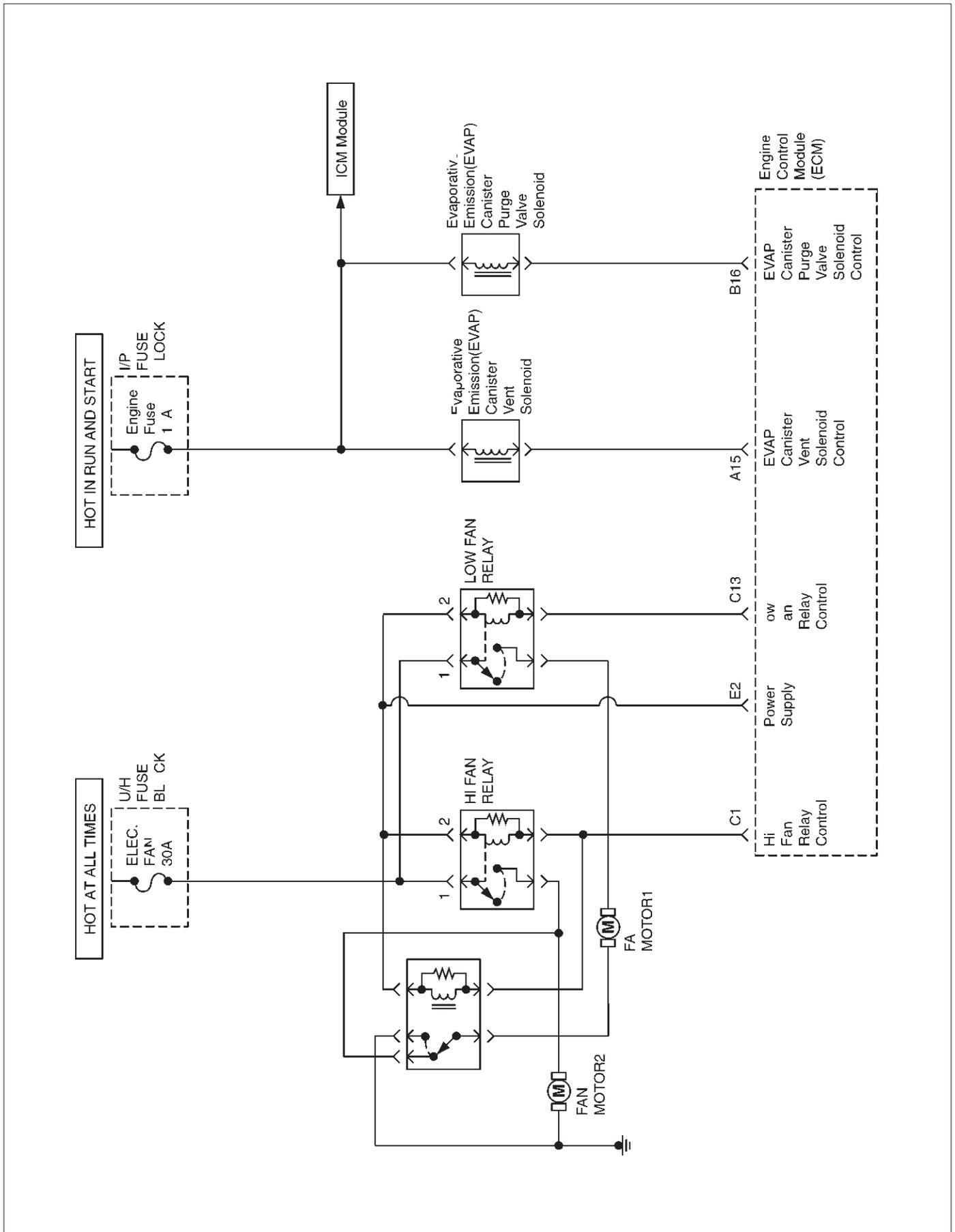
PCM WIRING DIAGRAM (8 of 13)
