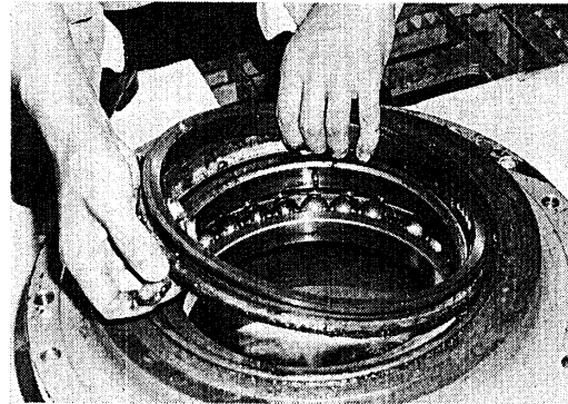
Fig. 33 Removing floating seal
