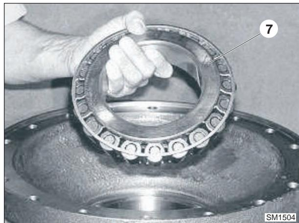
19. By using a puller and a metal stopper, turn the screw until the bearing outer ring (7) comes out.
