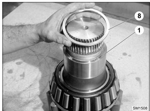
23. Position the pinion shaft (1) on the equipment (C) (xxxxxxxx). By using a press, take out the pinion shaft (1) from the bearing (4) and the nilos ring (3).
