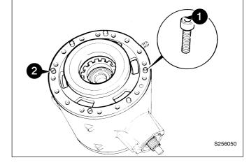
3 Drive out the differential side nut locking pin, to allow readjustment on assembly. Remove the other brake piston housing only if damaged, but remove its locking pin regardless (to allow sideload adjustment on assembly).
