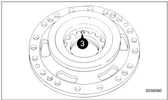
4 Lift out the crownwheel/differential assembly.
