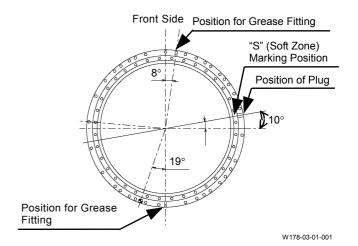
3. Install bolts (3) (36 used) to the inner race of the swing bearing and tighten to specification.
