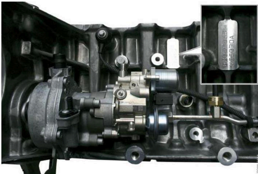
Fig. 3: Locating Engine Identification And Engine Serial Number - N55 Engine Courtesy of BMW OF NORTH AMERICA, INC.
