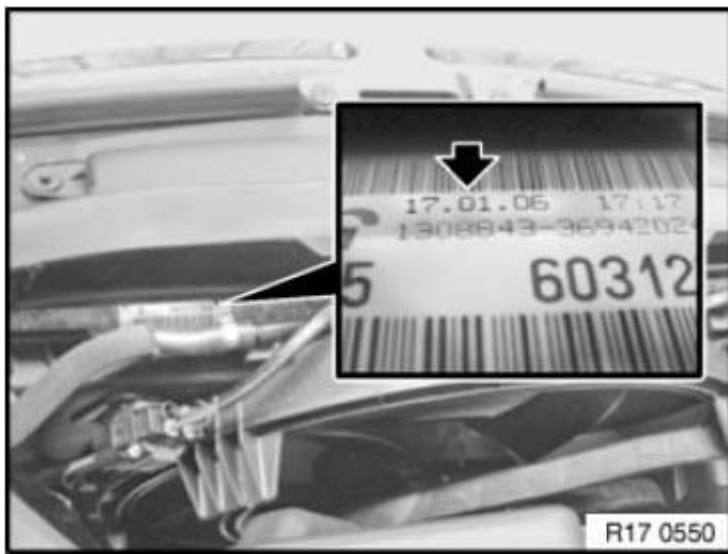
Fig. 4: Locating Production Date Courtesy of BMW OF NORTH AMERICA, INC.
