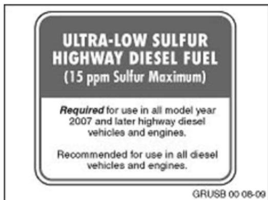
**Fig. 4: Identifying Ultra-Low Sulfur Highway Diesel Label**
