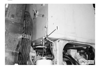
Install engine hood assembly. (For details, see INSTALLATION OF ENGINE HOOD ASSEM-BLY.)
